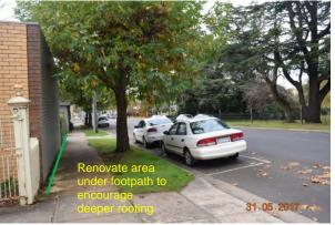
Figure 35: Option 1 recommended measures install root barrier (green) and renovate below ground space under footpath
