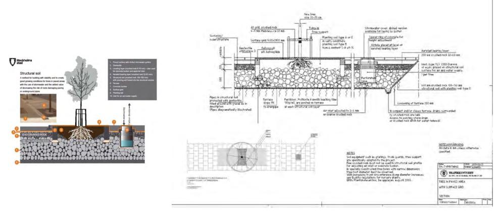
Figure 48: Stockholm structural soil system, an integrated approach to trees and infrastructure (City of Stockholm)
