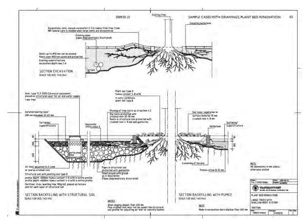
Figure 42: Renovation of planting area around large trees with a shallow root system (City of Stockholm 2009)
