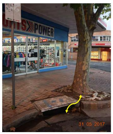
Figure 50: Future streetscape designs should integrate stormwater drainage and street tree planting pits to achieve multiple benefits
