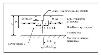
Figure 38: Dowelled control joint. Adapted from Sujeeva and Xie (nd).
